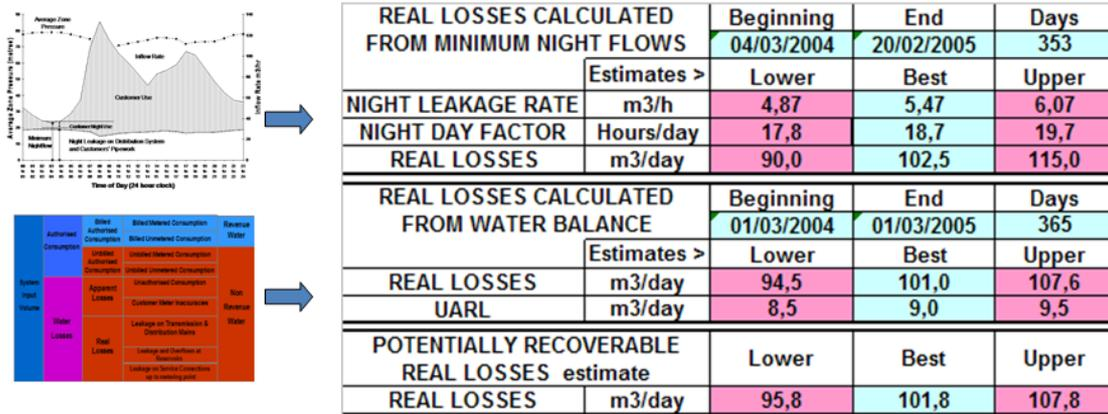
Figure 1.4 StiperzEnia Software comparing Real Losses calculated from Night Flows and Water Balance for a DMA in 2004 and in 2005
